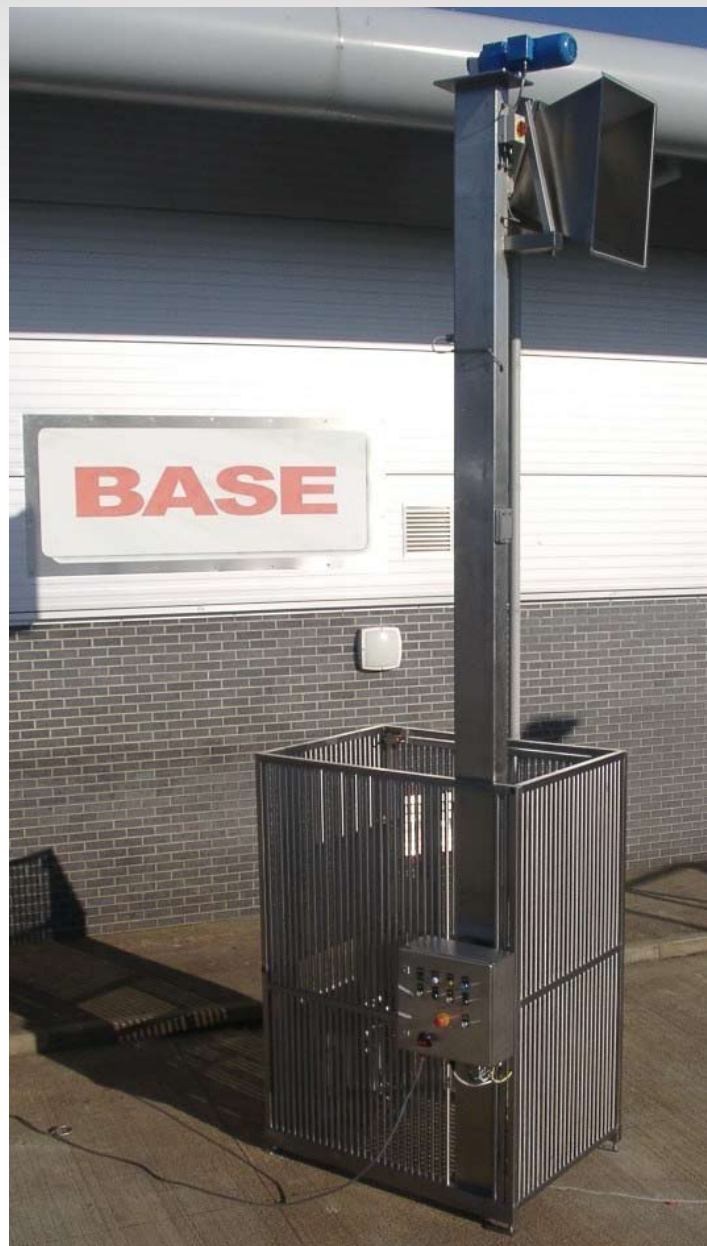
Single Pillar High Speed Tipper with Integral Skip
