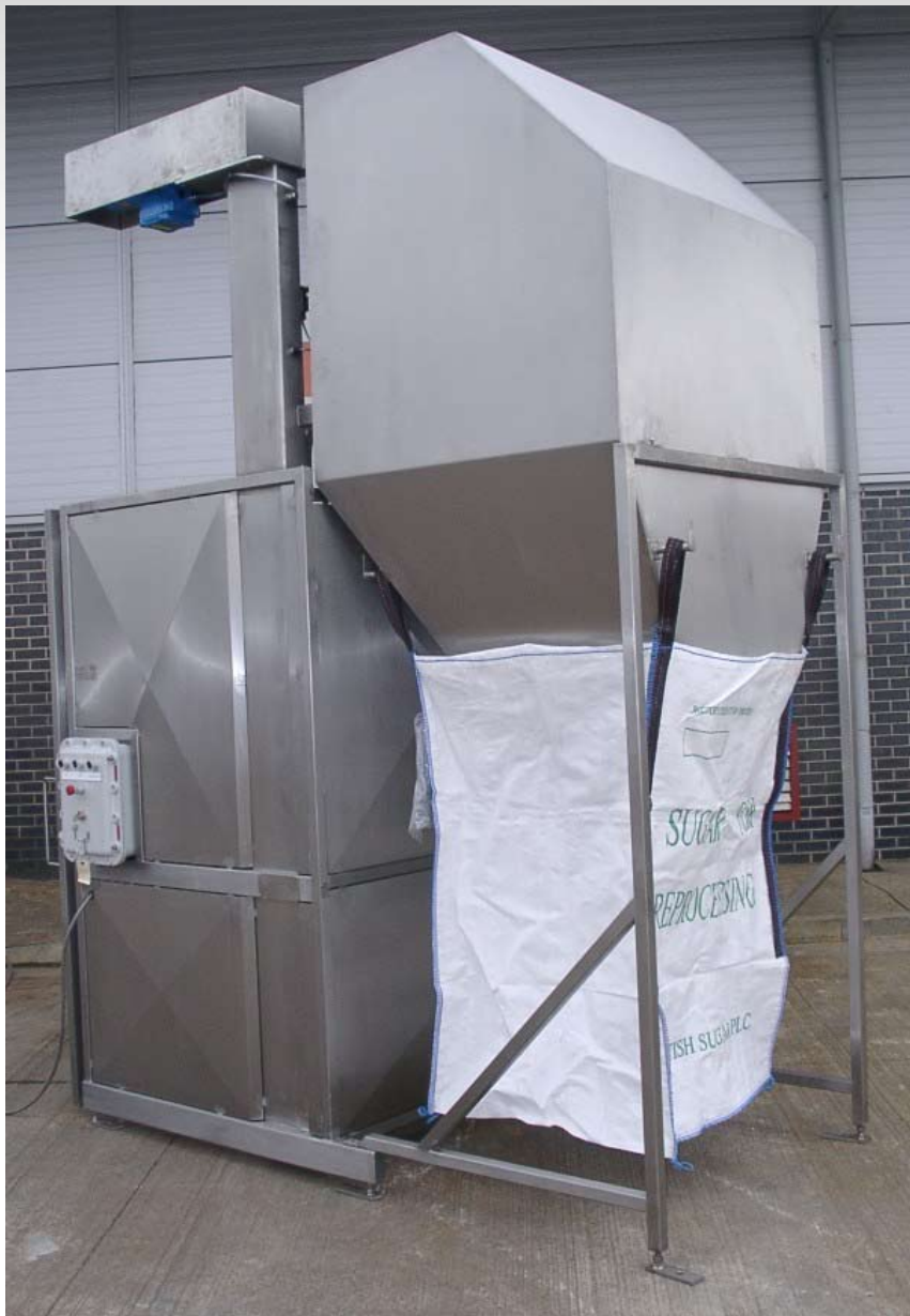
ATEX Bin Tipper for 200 Litre Tote Bin Bolted Guarded
