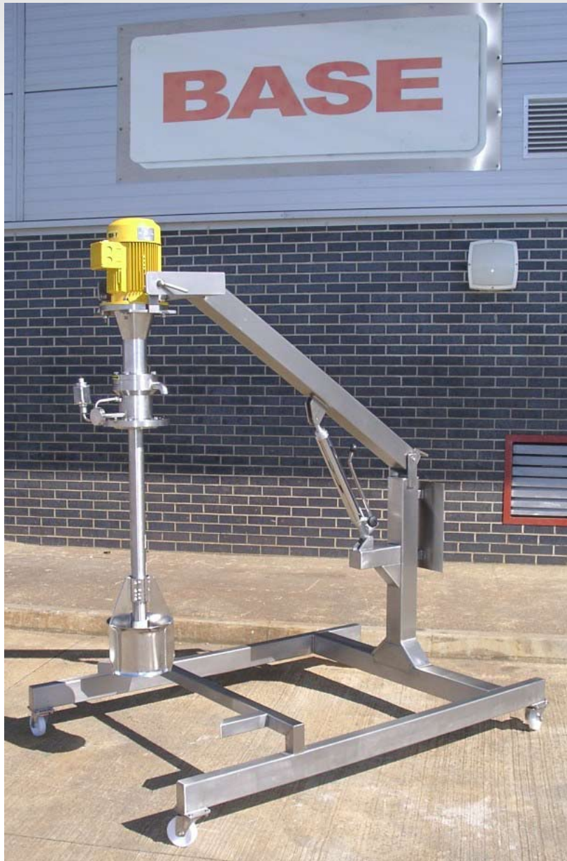
Hydraulic Mixer Lift
