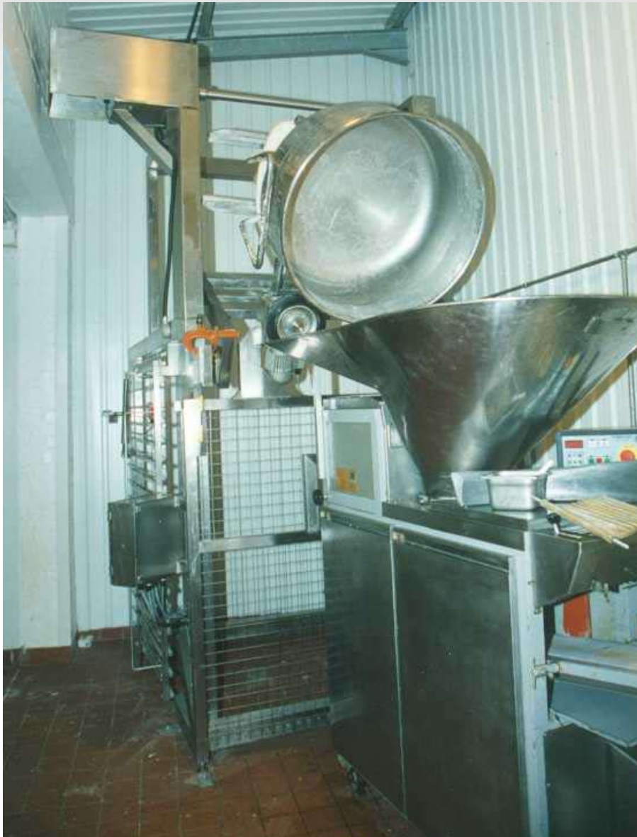
Double Pillar Mixing Bowl Hoist for Collette type Mixing Bowl
